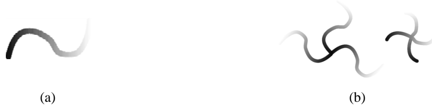
Figure 6. Example of a simple fuzzy line (a) and a (complex) fuzzy line (b). Fuzziness is indicated by shading. The complex fuzzy line consists of two fuzzy blocks that are made up of seven fuzzy simple lines.
