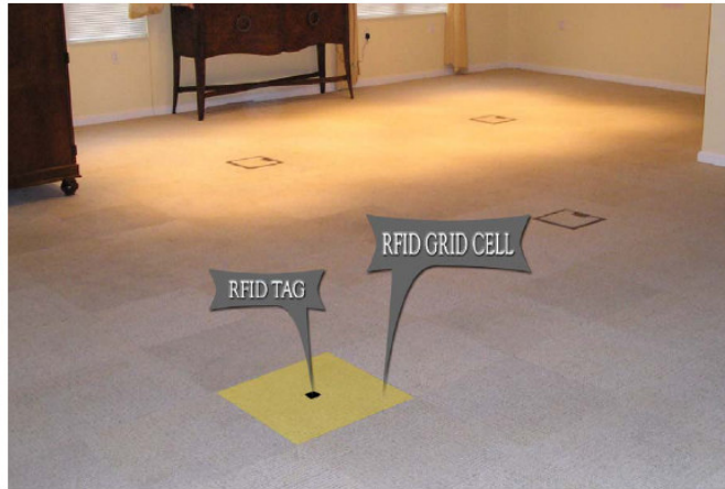
Figure 4. RFID grid in the GTSH
