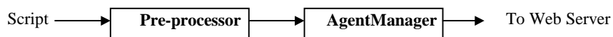
Fig. 1 Client-Side environment of the model. The script written in the restricted language of the model is run through a pre-processor and the syntax-error free script is parsed by the Agent-Manager . The AgentManager then moves to the first web server (as read from configuration)
