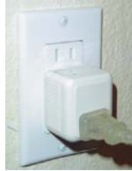
Figure 3. The smart plug used in the Gator Tech Smart House.
