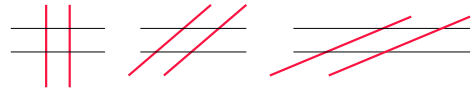
Figure 5. Area of parallelogram increases as angle between level curves decreases (top to bottom). Level curves of I_1 and I_2 are shown in black and red lines respectively.
